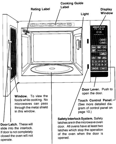
**Turntable.** Composed of glass tray and roller guide. The roller guide is placed first in the bottom of the microwave and supports the glass tray. Both parts must be in place when using the microwave.
